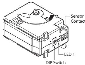
Example: With a current of 10 amps set as the threshold and a 15% differential, sensor contact will be closed between 8.5 amps and 11.5 amps and open outside of this range. A small amount of hysteresis is provided to prevent dithering near the differential limits.
